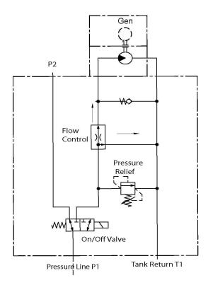
The HG hydraulic generator is a purpose built onboard hydraulic generator solution, designed specifically for the integration into existing hydraulic circuits. The unit shown above is suited to an extensive range of construction machinery that operate with fixed displacement pumps.
